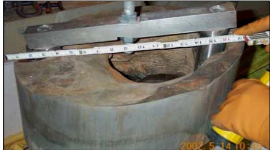
Nozzle #3 Area Cut Away From Reactor Head
