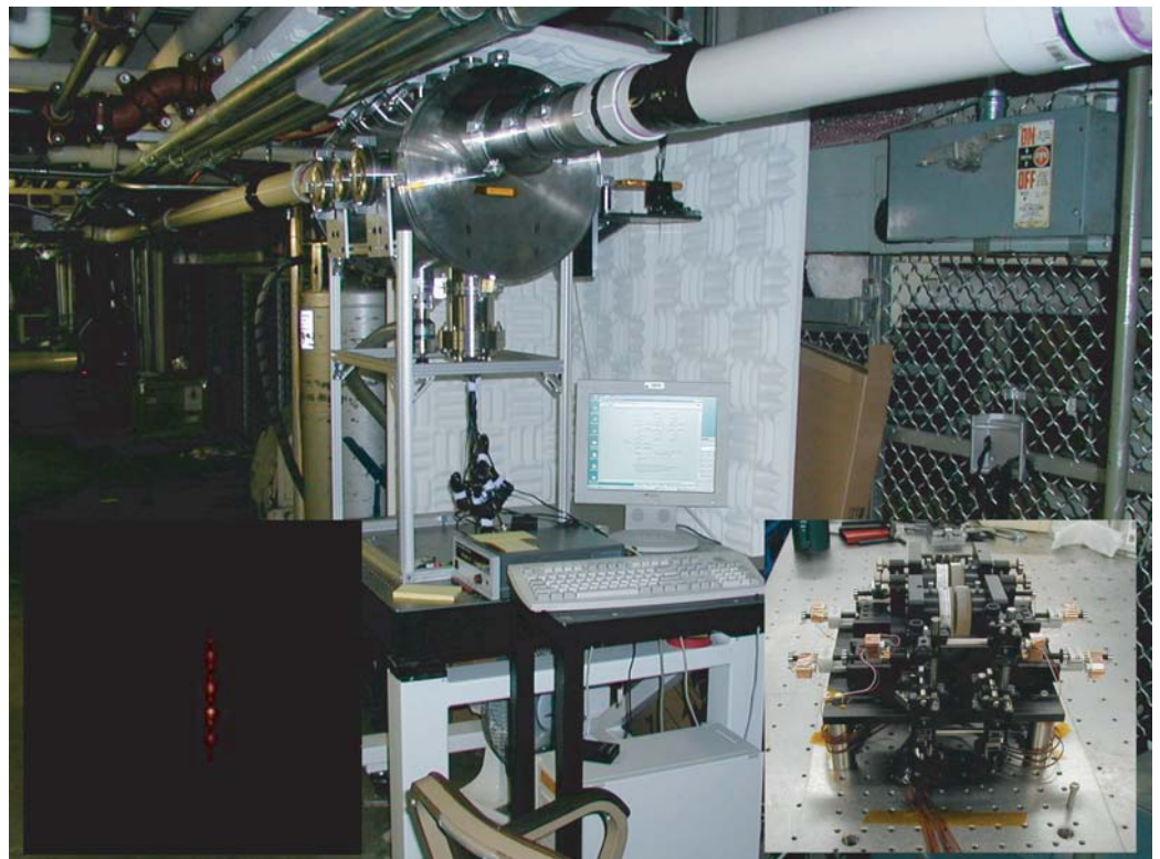
The Black Hole Imager makes use of X-ray interference (lower left), recently demonstrated in the laboratory.
