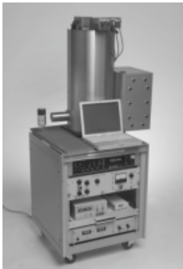
Fig. 4. Superconducting spectrometer (“UltraSpec”). \gamma -rays from the radioactive source on the left are detected by the TES detector held at \sim 0.1 K at the end of the cold finger. The signals are amplified at 4.2 K, readout with electronics in the enclosure on the right, and digitally processed.
