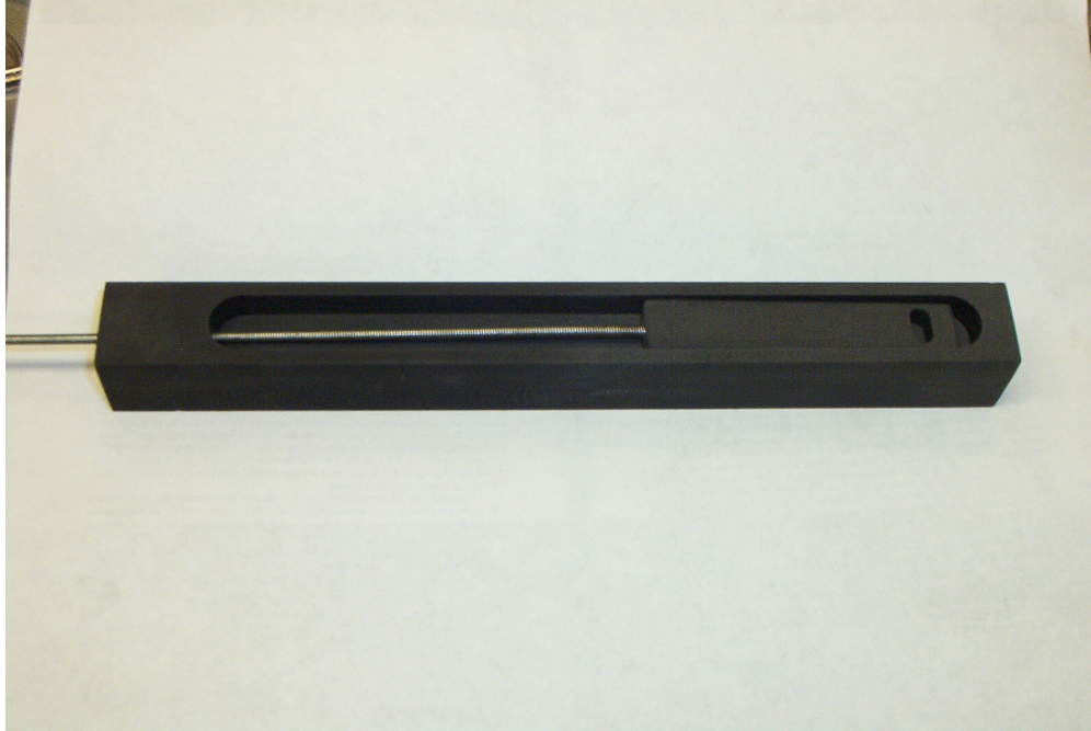
Figure 5: Sliding boat of the new sliding-boat reactor.
