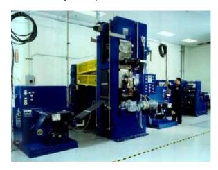
Figure 4.2 Calendering Machine (Source: Polystor Corp., Inc., 2000)
