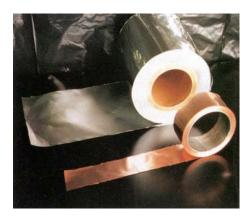
Figure 3.1 Current-Collector Foils (Source: Hohsen Corp. 1998)
