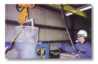
Figure 7.3 Toxco Cryogenic Freezing Process (Source: Toxco, Inc., 2000)
