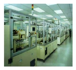
Figure 4.4 Automated Cell Assembly Line (Source: Polystor Corp., Inc., 2000)
