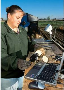
Technician Teresa Koppin checks sucrose content of a freshly harvested beet using a near-infrared instrument.
