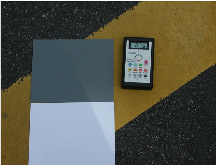
Figure 7 AltaII, Kodak gray cards on yellow thermoplastic over asphalt
