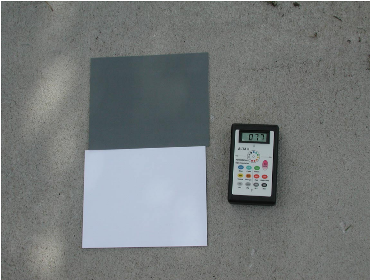
Figure 5 - Alta II, Kodak grey cards on concrete 3
