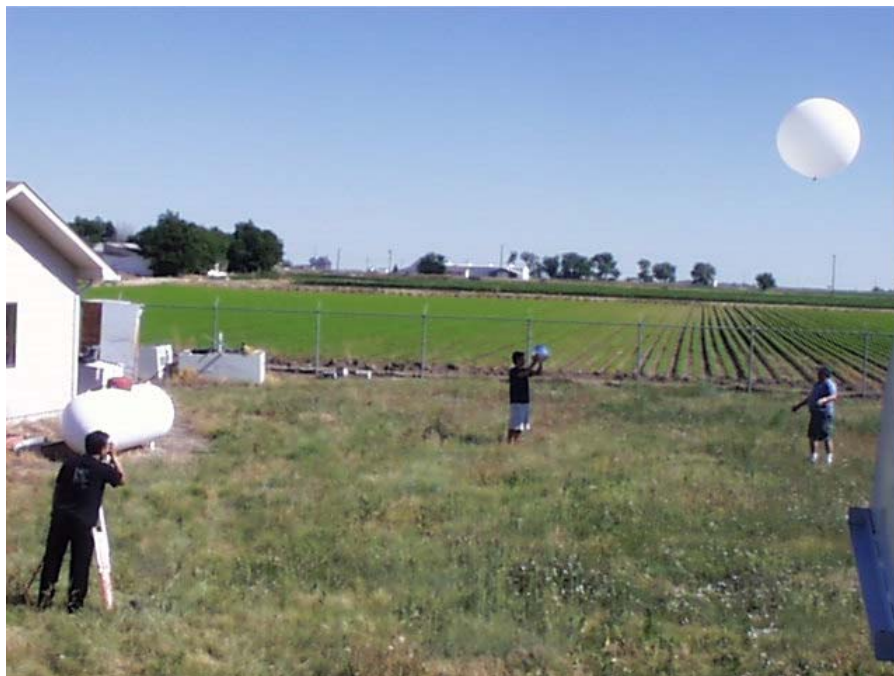
Figure 7 - Release of Radar Calibration Sphere from CSU-CHILL (Brunkow 2004)
