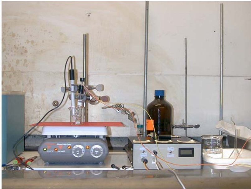
Fig. 4.5 Laboratory setup of the ORNL coulometric titration system
