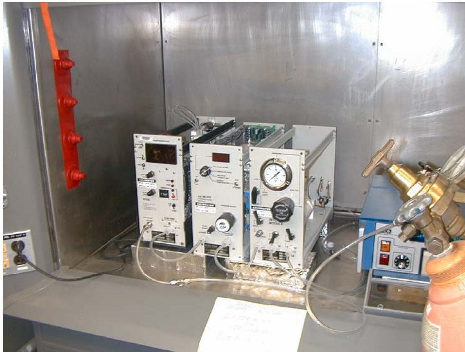
Fig. 3.2. Photograph of ORNL hydrazine gas generation/calibration system. From left to right: Gas mixer module, humidifier module, and interface module. The MDA 7100 sits on the far right, close to the gas cylinder.
