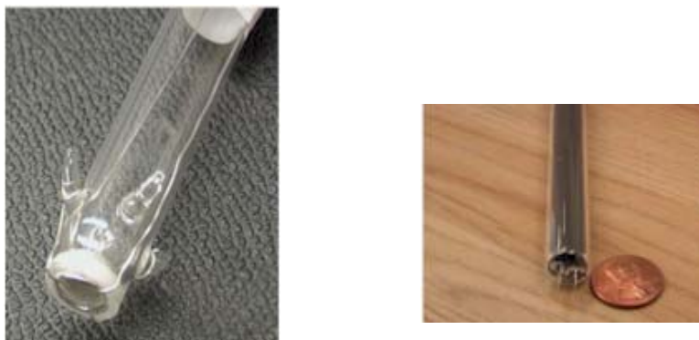
Fig. 4.2 Bromine generator electrode (left) and sensing electrode (right). The two electrodes are approximately the same size, but the top electrode has been exaggerated to show the design.
