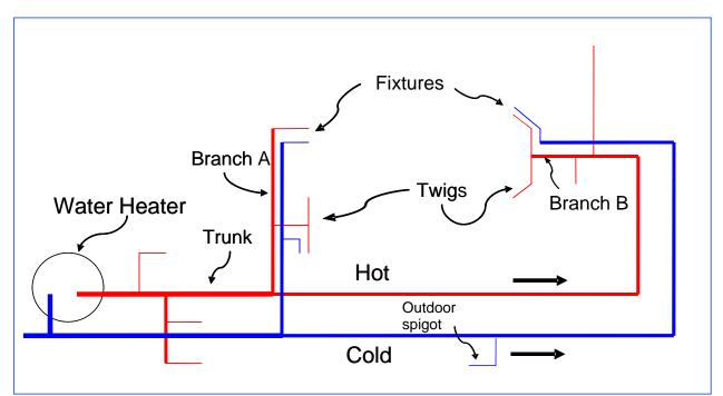
Figure 1: Conventional Single Trunk, Double Branch and Twig Plumbing Layout with Separate Hot and Cold Water Supply Lines to individual fixtures.
