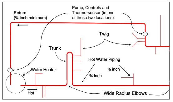
Figure 3 Structured Plumbing System with a Dedicated Return Line
