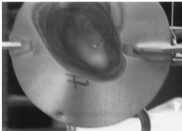
FIG. 19. Picture of a metal plate heated by a propane torch from its back surface.
