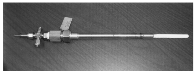
FIG. 11. BeO combustion gas temperature probe.
