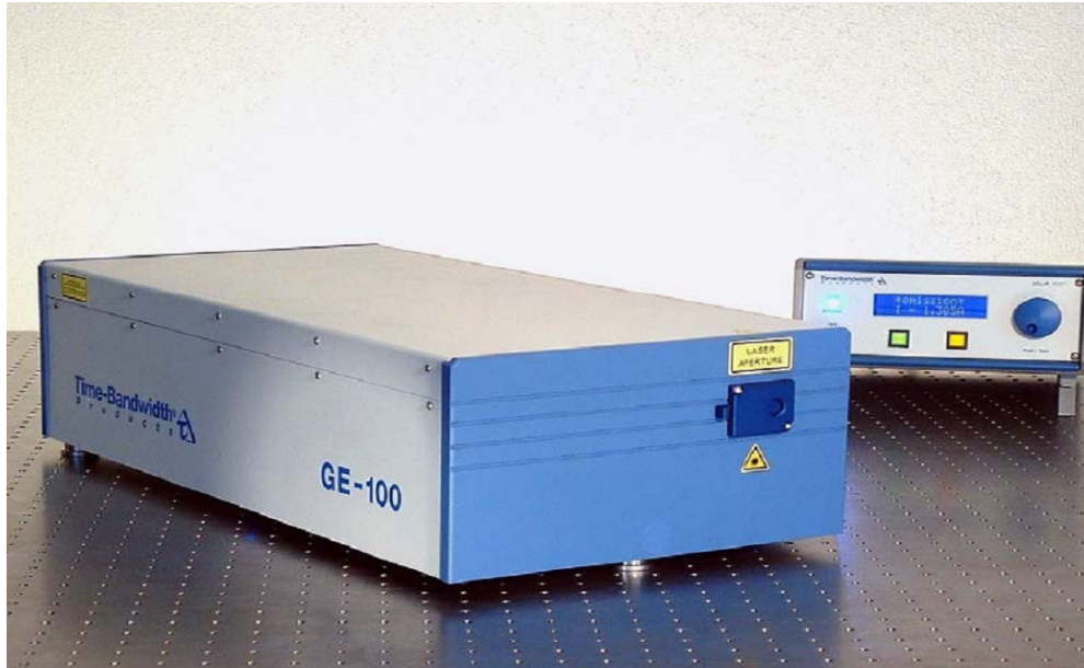
Figure 2.2: A photograph of a new seed laser purchased from Time-Bandwidth, model GE-100 (Nd:YLF, 0.5 W, 5 ps, \lambda=1054 nm).
