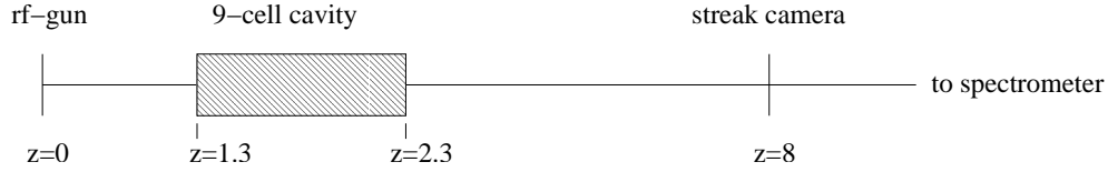
Figure 4.2: Simplified block diagram of the A0 beamline.
