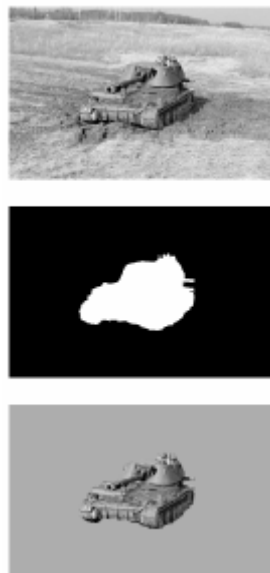
Figure 1. Construction of an apertured image. A) Original image, B) aperture, C) apertured image.
