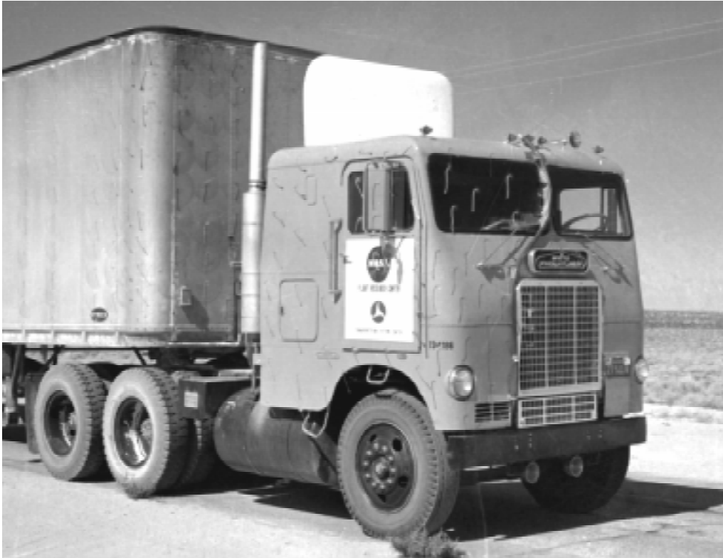
(c) Cab-over-engine tractor and semitrailer with cab-mounted add-on device.
