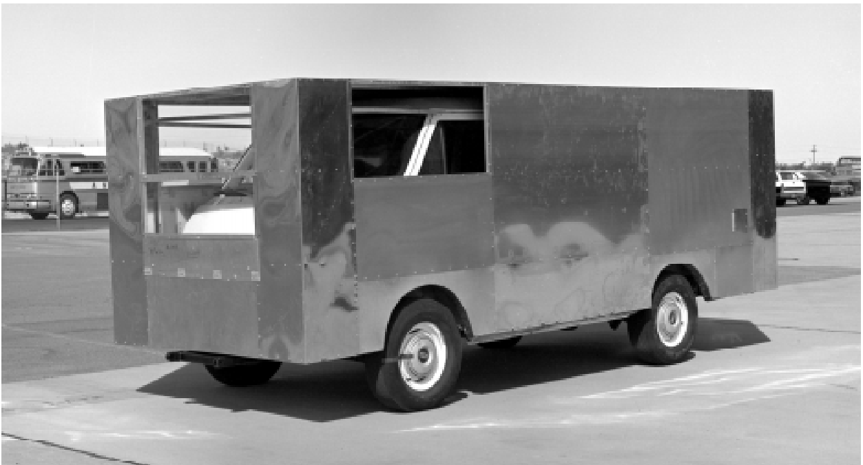
(b) Test van configuration A (all square corners).
