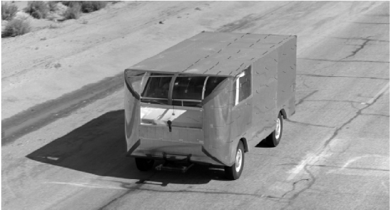
(c) View showing attached-flow tuft pattern on upper surface when front corners are rounded.
