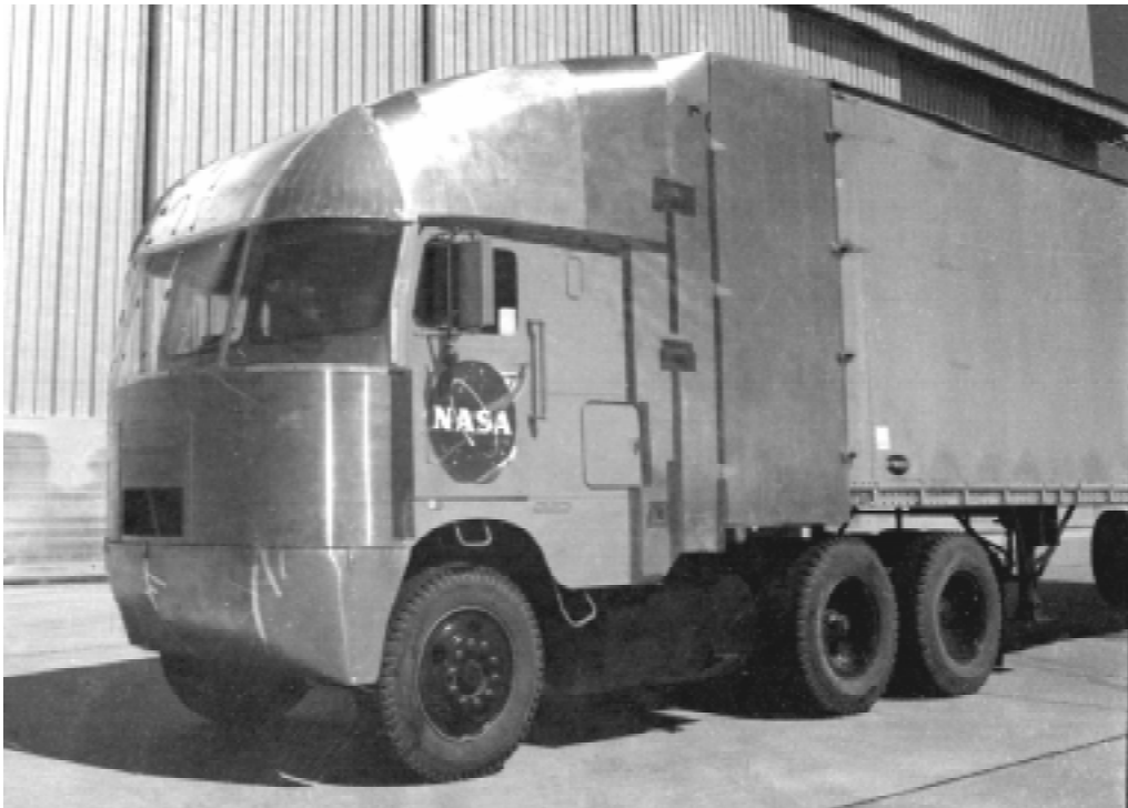
(d) Low-drag cab-over-engine tractor-semitrailer configuration.
