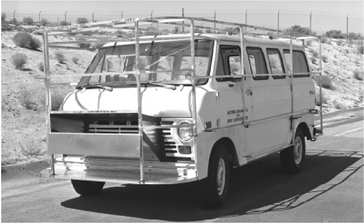
(a) Partly constructed test van showing substructure.
