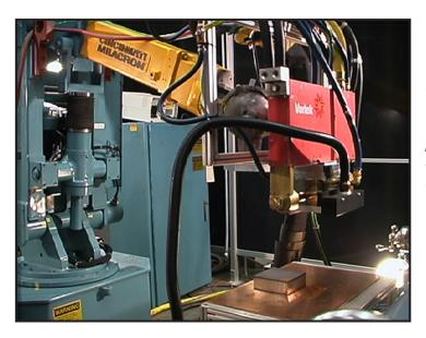
ORNL's process for metallurgical bonding of high-performance refractory metal coatings uses the world's most powerful plasma-arc lamp, shown here on a robotic control arm, to project high-intensity infrared energy.
