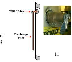
machine is "low" or "high" temperature. A TPR valve is also present on the booster heater supplying hot sanitizing rinse water to "high temp" machines. TPR valves have a limited service life and will eventually fail.
