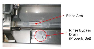
Rinse nozzles should also be regularly inspected for wear. Worn rinse nozzles with larger openings will result in greater water consumption during the rinse cycle.
