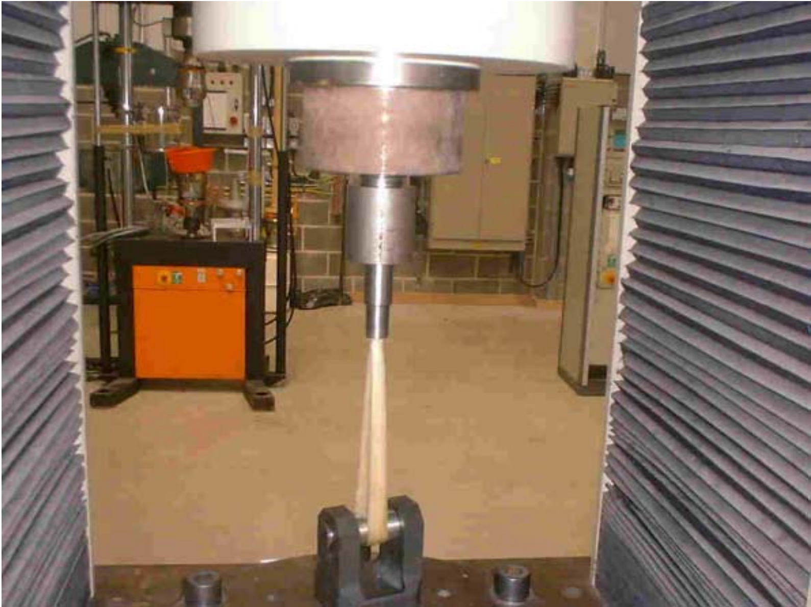
Portions of Cryomagnet Support Strap Undergoing Static Testing
