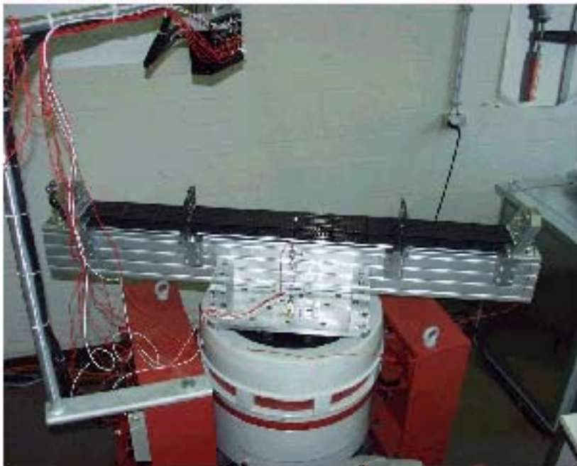
49" Module Vib Test No Radiator Material
