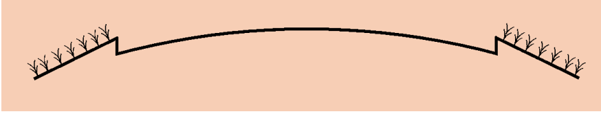
Roadway with parabolic crown. The outer edge of the road slopes too much. Gouging causes high shoulder, and center 1/3 of the road tends to be flat.
