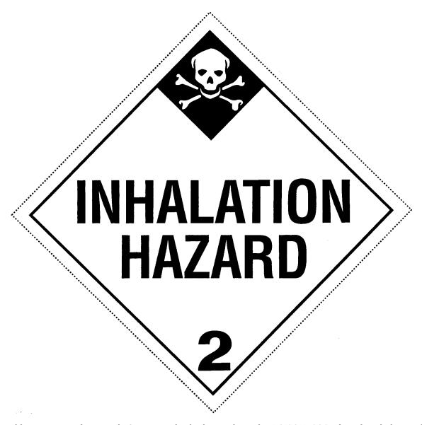
(b) In addition to complying with § 172.519, the background on the POISON GAS placard and the symbol must be white. The background of the upper diamond must be black and the lower point of the upper diamond must be 65 mm ( $2^{5}$ /s inches) above the horizontal center line. The text, class number, and inner border must be black.
