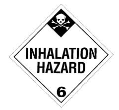
(b) In addition to complying with §172.519, the background on the POI-SON INHALATION HAZARD placard and the symbol must be white. The background of the upper diamond must be black and the lower point of the upper diamond must be 65 mm (2% inches) above the horizontal center line. The text, class number, and inner border must be black.
