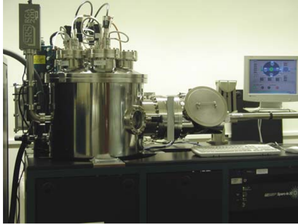
Figure 1.—The deposition chamber, load lock, and computer interface of the ATC2000 Sputtering System (#AJA1825).
