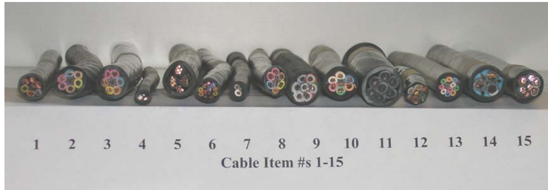
Figure 3.8: Photograph of the 15 different cables tested in CAROLFIRE.
