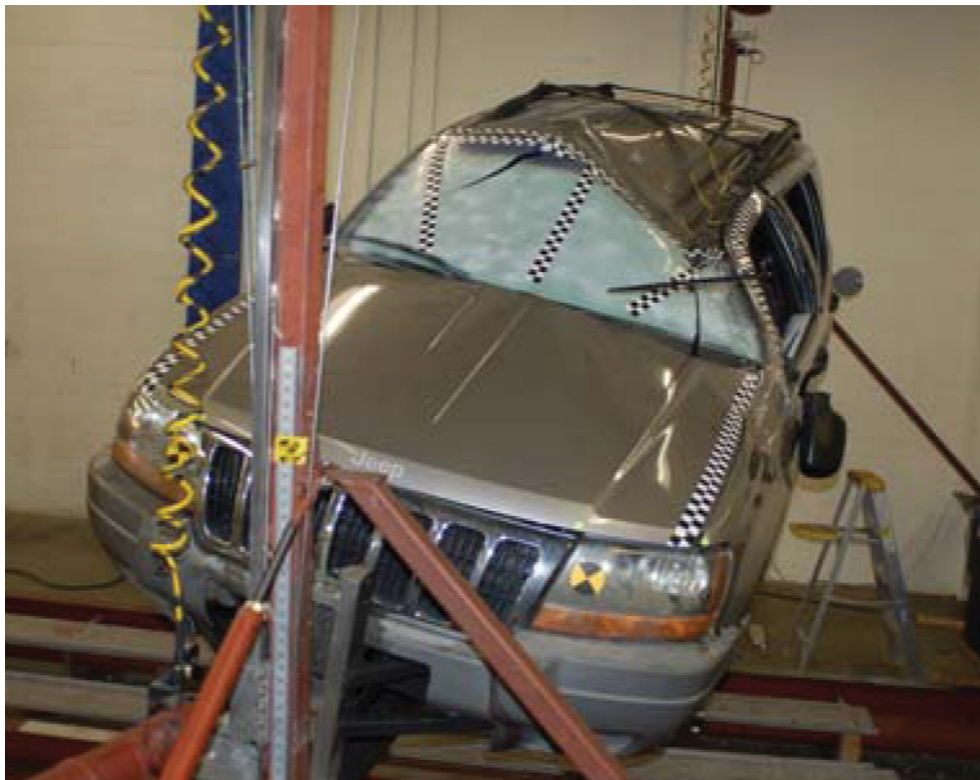
Figure 2 showing 1999 Grand Cherokee with roof buckle
