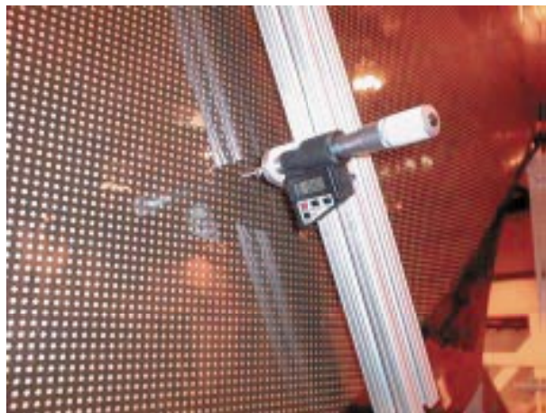
Fig. 8. The trammel arm/caliper system used to measure the flatness of the reflectarray membrane: (a) trammel arm and (b) caliper with digital readout.
