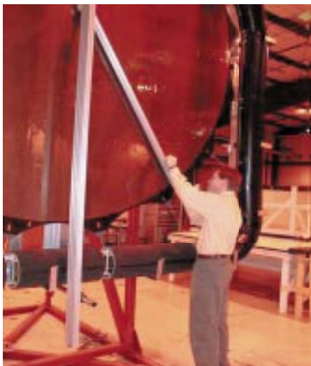
Fig. 8. The trammel arm/caliper system used to measure the flatness of the reflectarray membrane: (a) trammel arm and (b) caliper with digital readout.
