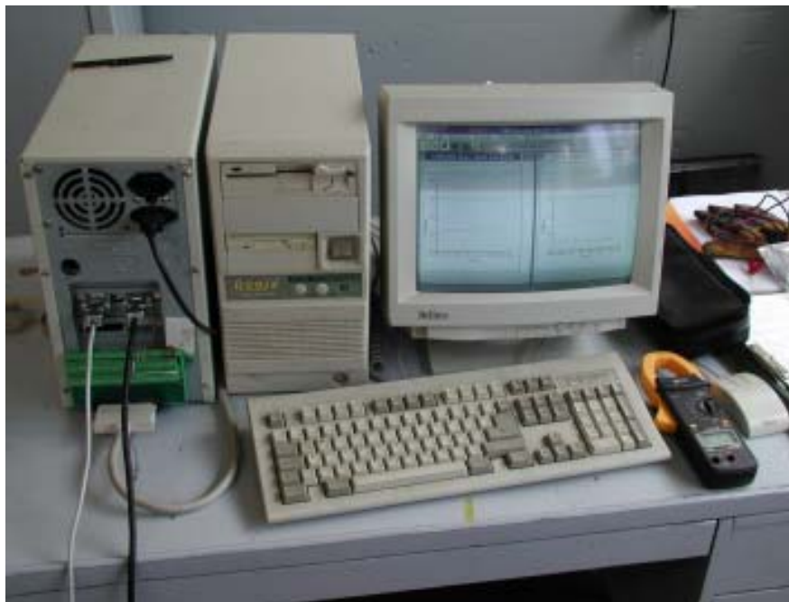
Figure 2. Photo of the on-line arc-welding monitor.
