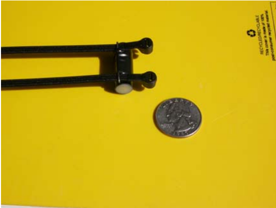
Plastic cable tie harness holding a micro sonic transmitter.
