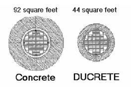
Fig. 2. Comparative diameters of concrete and DUCRETE<sup>™</sup> dry-storage cask or silo. Using DUCRETE<sup>™</sup> in an SNF cask or silo reduces the weight by 30%, the footprint by 50%, and the diameter from 132 in. (3.5 m) to 90 in. (2.3 m).
