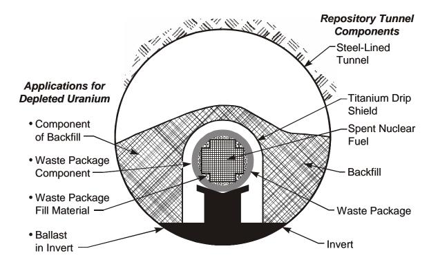
Fig. 1. Potential depleted uranium dioxide applications in a spent nuclear fuel geologic repository.
