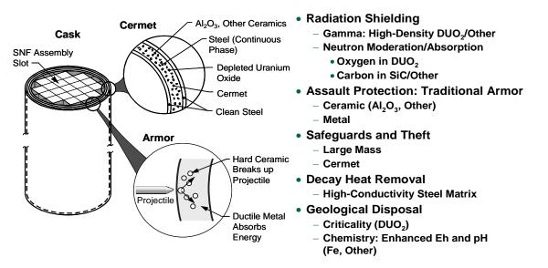
Fig. 3. SNF casks made of cermet (ceramics embedded in steel).
