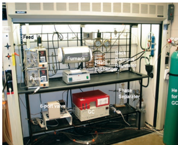
FIGURE 1. Reactor for the Production of Hydrogen by Reforming in Supercritical Water
