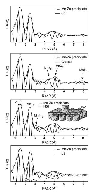
Fig. 4. Fourier transforms (FTs) of the *k*-weighted Mn-EXAFS spectra for the Mn–Zn precipitate (dotted lines) and synthetic <sup>VI</sup>Zn-sorbed  $\delta$ -MnO<sub>2</sub> (dBi), chalcophanite (Chalco), hexagonal birnessite (HBi), and lithiophorite (Lit). E and TC subscripts denote Mn–Mn contributions from octahedra linked by edges and triple-corners, respectively.
