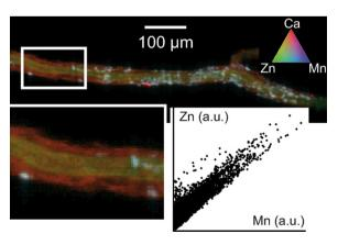
Fig. 2. Tricolor (RGB)  $\mu$ -XRF map of a root with Mn–Zn precipitates. Red codes for Ca, green for Zn, and blue for Mn. Each pixel is colored in proportion to Ca-, Zn- and Mn–K $\alpha$  signals. Pixel size is 7 × 7  $\mu$ m<sup>2</sup>. The graph is a pixel-by-pixel scatterplot of Zn counts vs. Mn counts, showing the constant Zn:Mn ratio.
