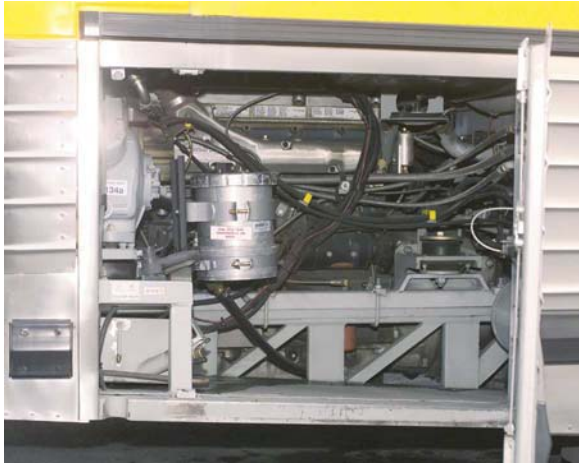
Figure 9. View of the bypass filter in the passenger-side engine compartment of a bus with a Series 60 Detroit Diesel engine.
