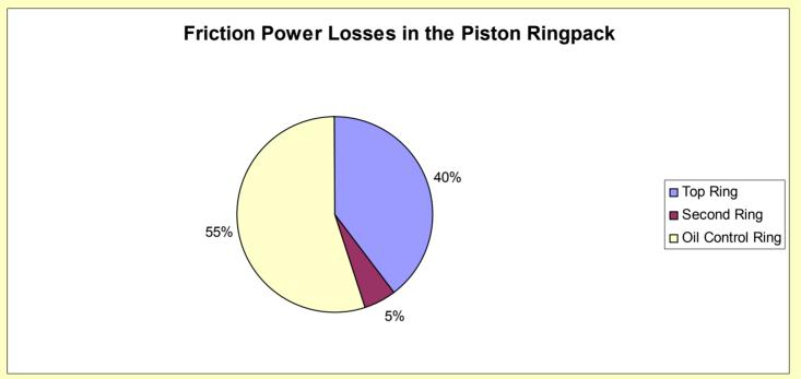
> Top ring and oil control ring are main contributors to friction in ringpack
