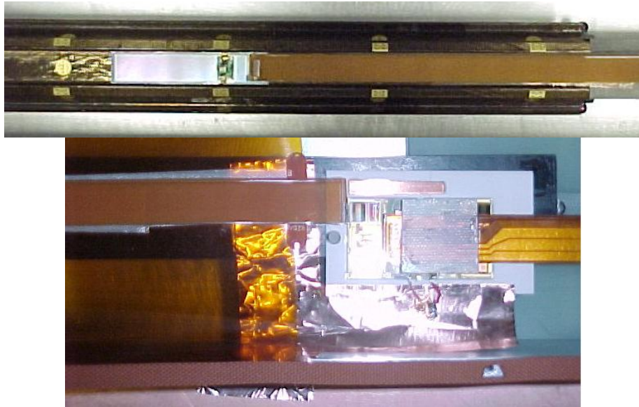
Figure 1: Top: Photograph showing the sensor part installed on the L0 support structure. Bottom: Photograph showing the hybrid part installed on the carbon fiber extension.
