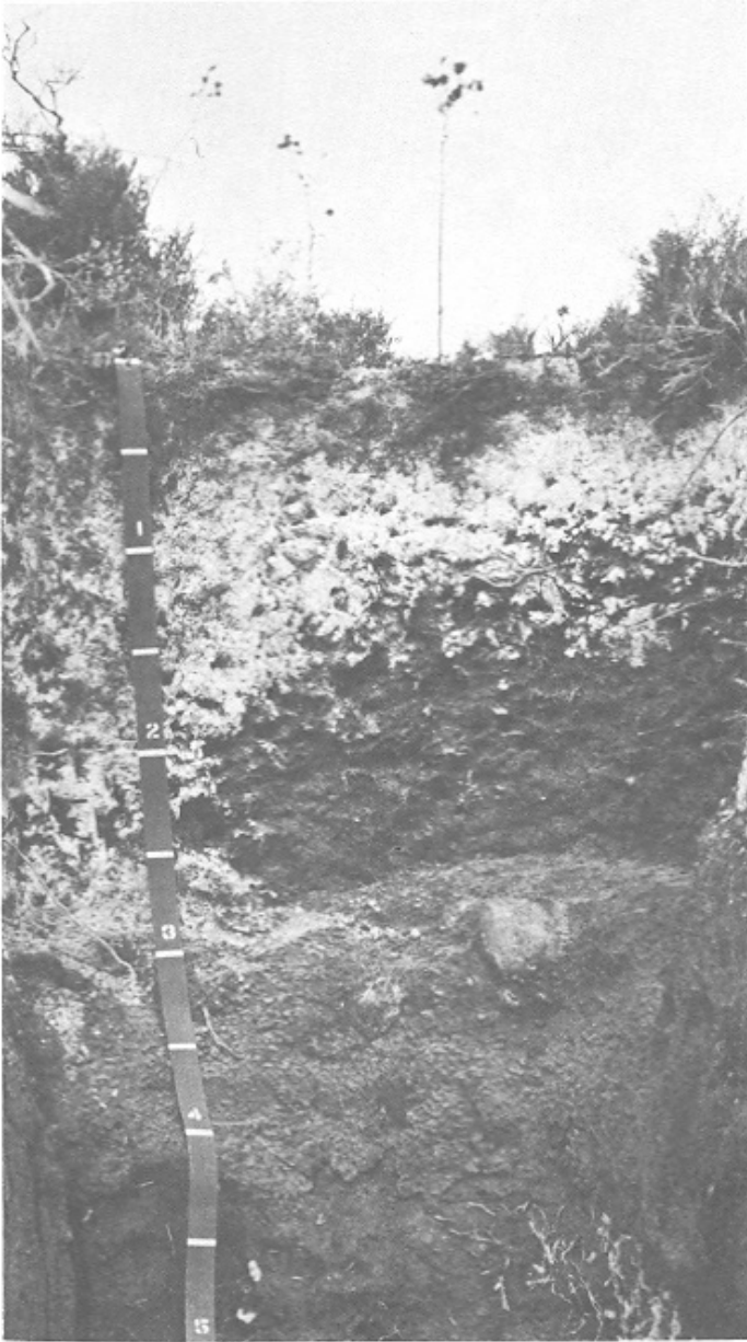
Figure 7.-Soil profile of Abo Variant loam. White crusting is salt.
