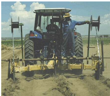
Figure 5. Tape installation with modified “Ox” ripper implement.
