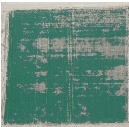
Figure 12. Field in 2002 showing further degradation of emitters due to root intrusion.
