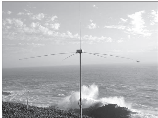
CODAR-type HF radar antenna deployed along the coast south of Monterey
