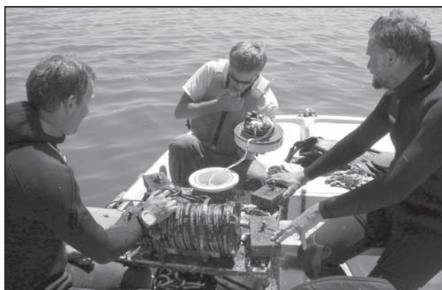
Nick Nidzieko prepares an acoustic Doppler current profiler for deployment at LOBO2 with the help of his assistants Jim Hensch (left) and Stephen Monismith (right).
