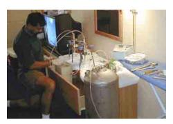
Filtration of water samples from the Eel River. Water samples were filtered for polycyclic aromatic hydrocarbons (PAHs) by pressurizing the sample vessels with ultra-high-purity nitrogen. The exit line of the pressure vessel was connected to a 142-mm-diameter stainless-steel filter holder housing a precleaned glassfiber filter. Additional water samples were simultaneously filtered for black carbon.
