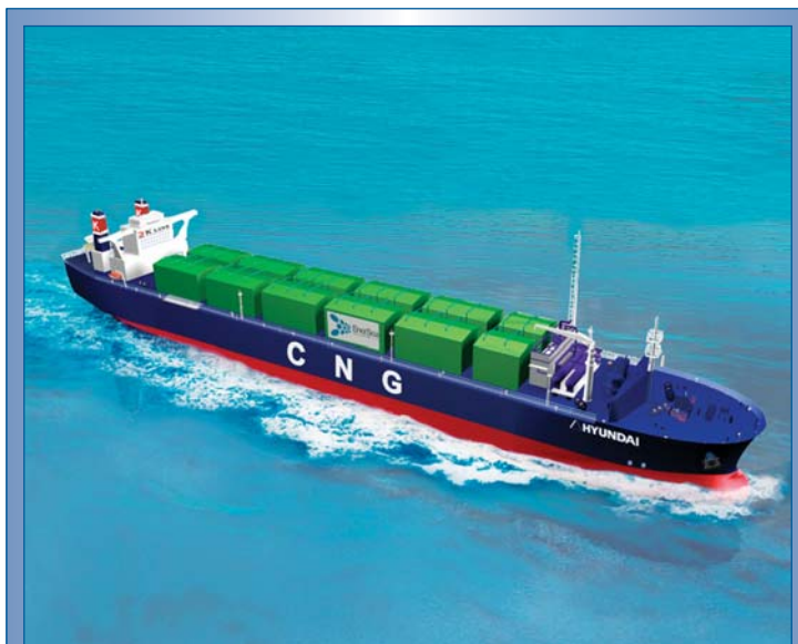
Figure 1. EnerSea Transport's V-800 compressed natural gas carrier.
