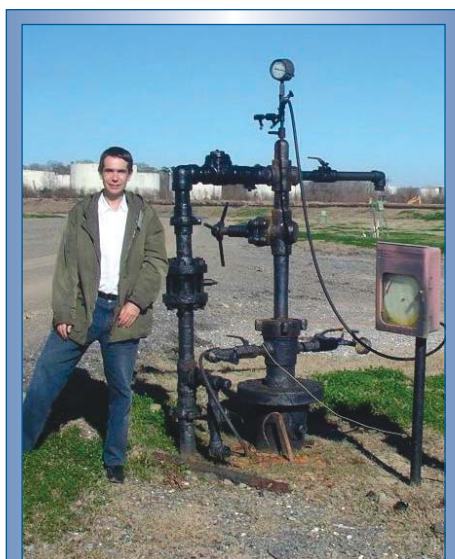
Figure 3. A Class II injection well (Photo by J. Veil, Argonne National Laboratory)
