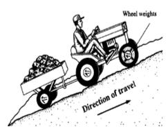
Figure 4. Downshift to a lower speed when climbing steep grades. Loads on the rear increase the chance of backward upset. Add front wheel weight for balance.
