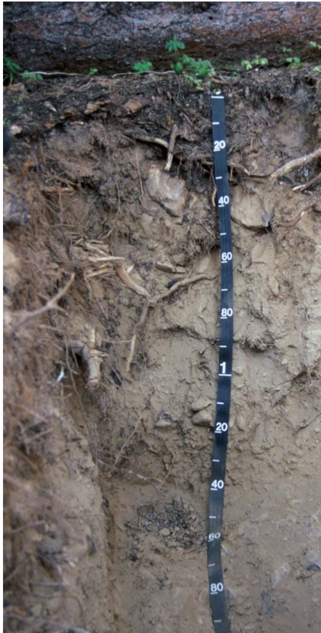
Figure 13. —Typical profile of an Oatman soil. A duripan is at a depth of about 140 centimeters. Measurements on tape are in centimeters.
