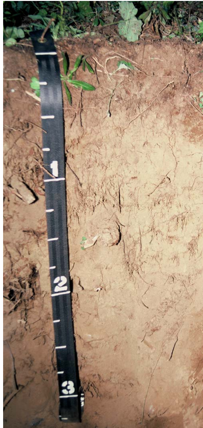
Figure 10.—Typical profile of a Grousehill soil. Measurements on tape are in feet.
