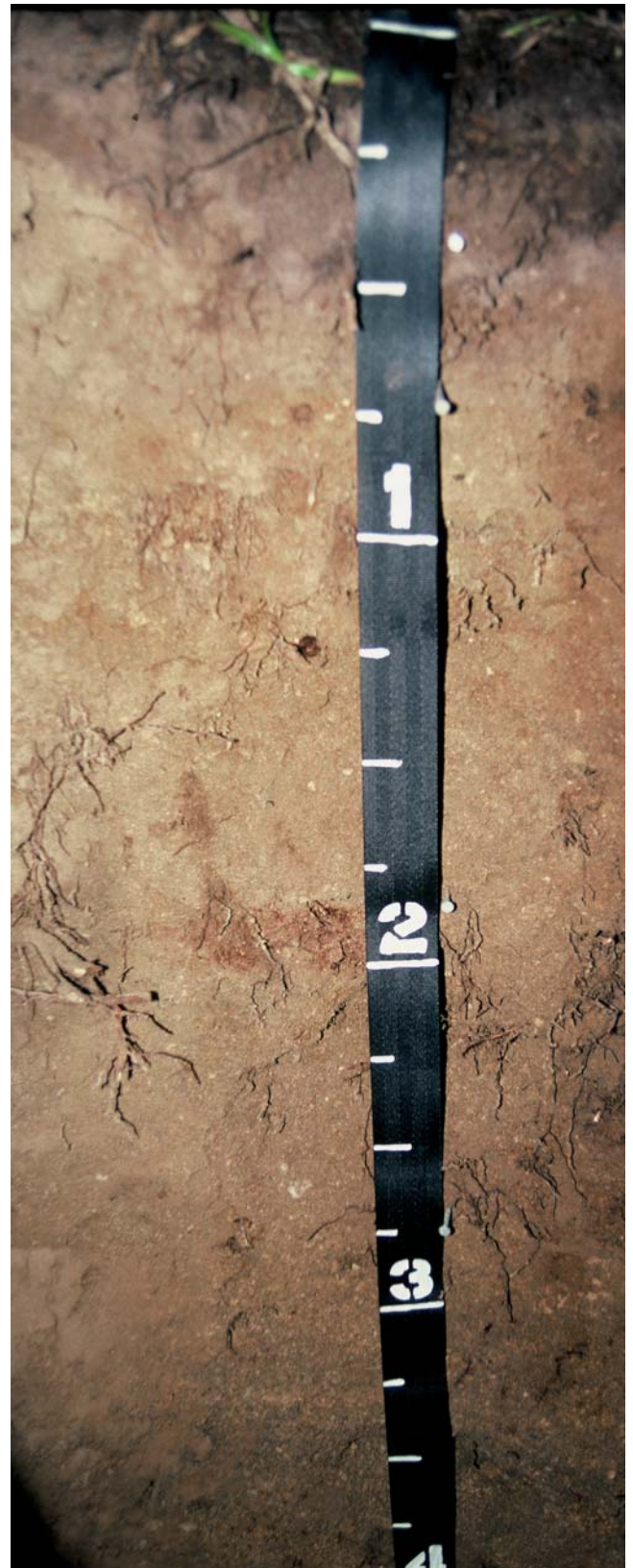
Figure 8.—Typical profile of a Castlecrest soil. Note the white, discontinuous E horizon at a depth of about 4 inches. Measurements on tape are in feet.
