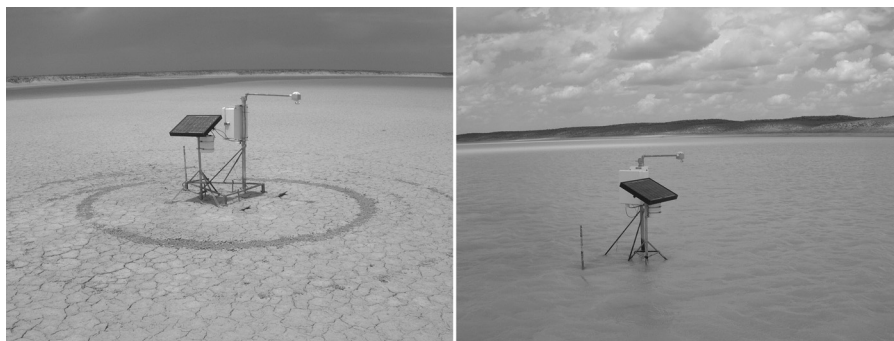
Fig. 4. The acoustic water level sensor. Water depth is determined by measuring the time it takes for a sound wave to bounce off the water surface and return to the sensor.
