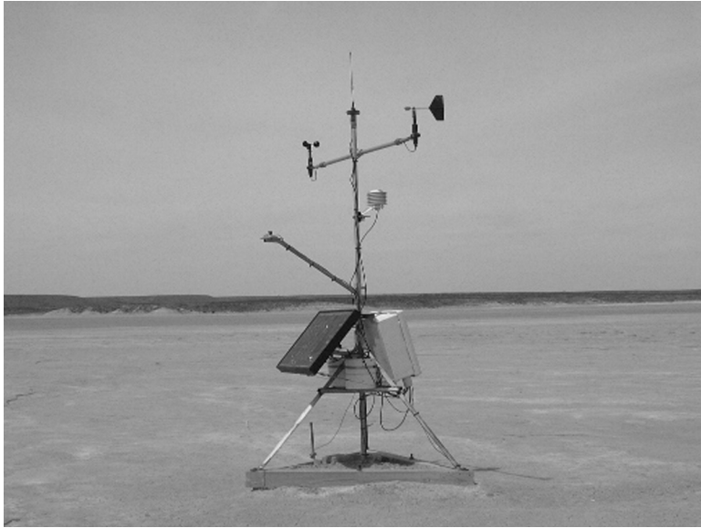
Fig. 5. The 2-m meteorological tower equipped with an anemometer, wind vane, pyranometer, relative humidity, and temperature sensors.
