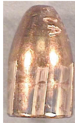
Figure 1-5: Fired bullet showing land impressions.
