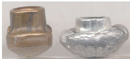
Figure 2-3: Fired bullets mushroomed by impact; note the visible land impressions at the base of each bullet.
