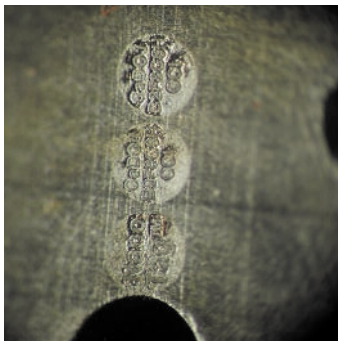
Figure 3-3: Breech face marked with redundant microstamps. (ID Dynamics, LLC [NanoVia Ballistic Program Acquisition])
