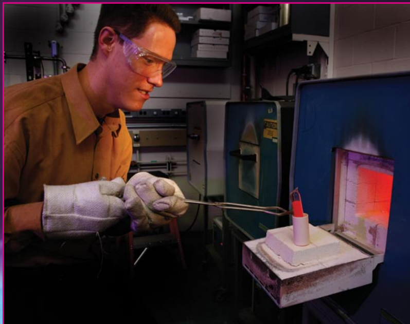
Los Alamos scientist Eric Bauer heats a small metal sample to 1600 degrees Fahrenheit as the starting point for growing large single-crystal samples of unconventional superconductors.
