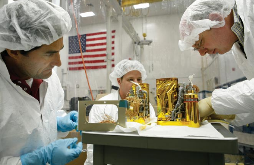
One of Cibola's radio antennas during the satellite's testing phase. Once Cibola was in orbit, a 2.3-meter-long antenna successfully deployed from the gold-colored canister.
