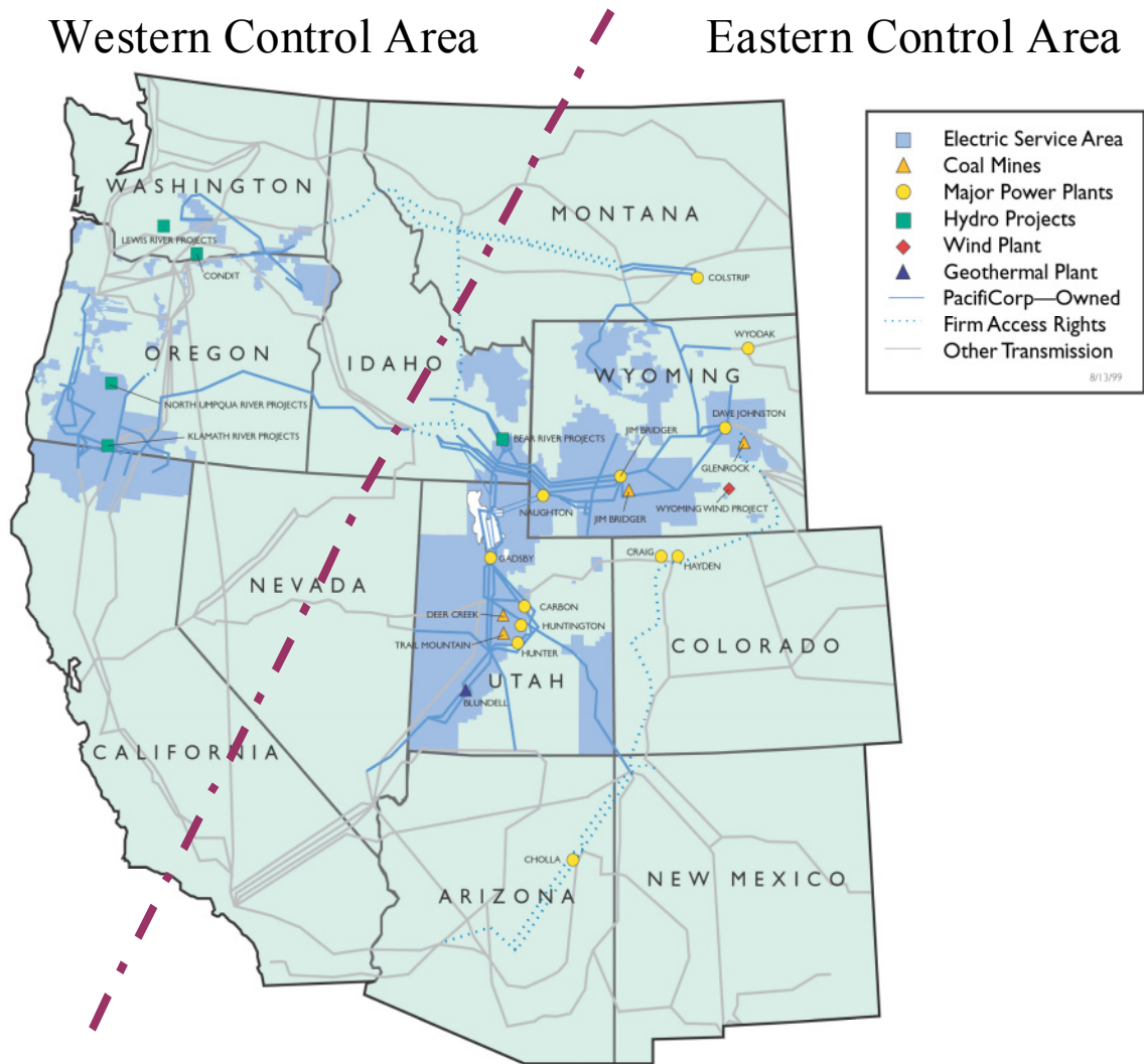
FIGURE 4. PACIFICORP POWER SYSTEM MAP AND CONTROL AREA.
