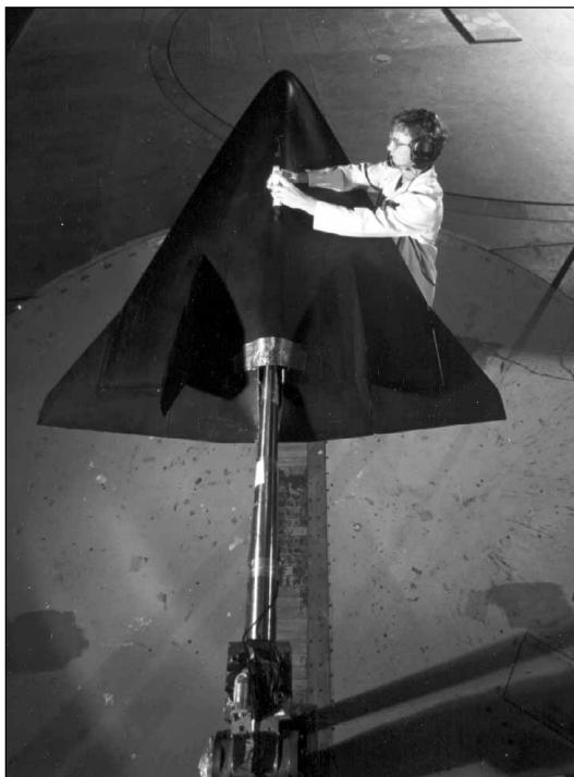
An Engineer determines the inclination of a LoFlyte™ Wind Tunnel Model.
