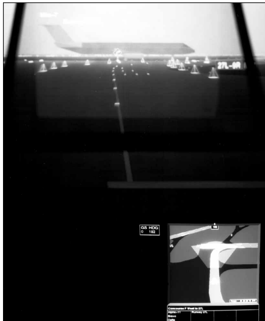
T-NASA's Head-Up Display (HUD) shows cleared taxi route using virtual reality.
