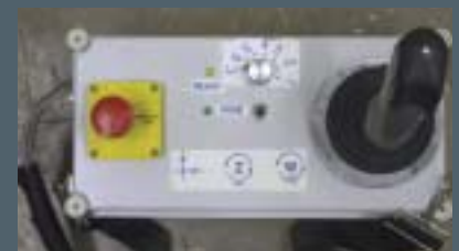
Operator uses a joystick to manoeuvre the Flying Carpet. The joystick mimics some of its movements: push the joystick forward and back and side to side to move along the Y and X axes. Twist the joystick to move up and down (marked Z). The odd one out: yaw. To pivot along the vertical axis, operators press and hold a thumb button (not visible) and twist. The control also includes a red emergency stop button and a hoist set-up dial
