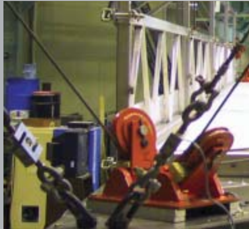
Two cables terminate at each corner of the Flying Carpet. Cable runs start at the hoist's rope drum, then travel through pulleys located near the anchor point, loop around a snatch block, and then fastens to the Flying Carpet through an S-shaped load cell
