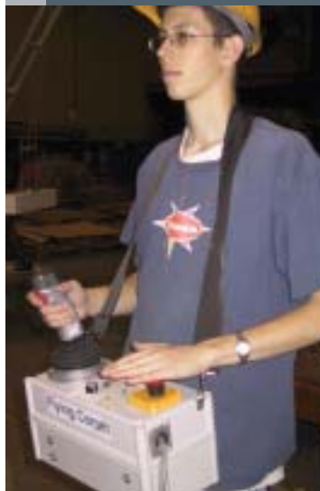
Operator uses a joystick to manoeuvre the Flying Carpet. The joystick mimics some of its movements: push the joystick forward and back and side to side to move along the Y and X axes. Twist the joystick to move up and down (marked Z). The odd one out: yaw. To pivot along the vertical axis, operators press and hold a thumb button (not visible) and twist. The control also includes a red emergency stop button and a hoist set-up dial
