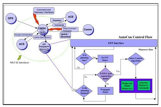
Figure 3. EO-1 EFF Functional Diagram (GSFC Approach)
