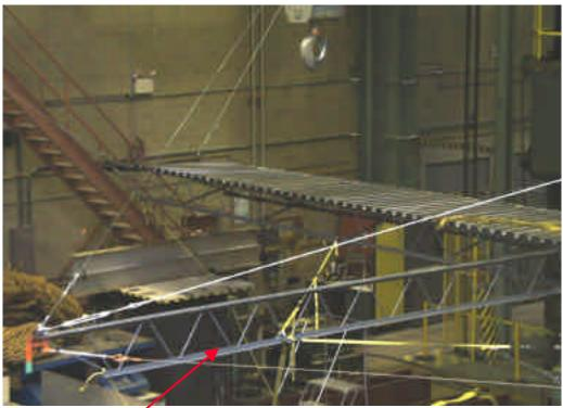
Stabilizer/Rotator provides rigid support and yaw rotation of platform.
