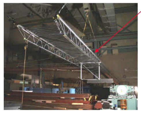
Large, suspended platform can be position controlled using proven RoboCrane joystick-control technology. View from beneath platform
