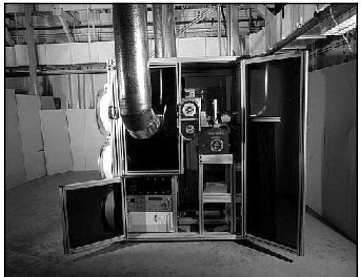
The Radionuclide Aerosol Sampler/Analyzer (RASA) unit can be used to confirm nuclear detonations anywhere in the world.
