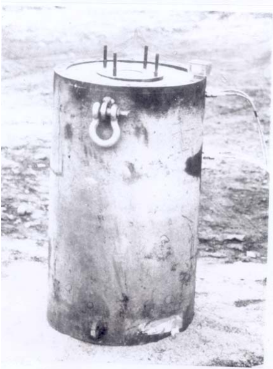
Fig. 5. Photograph of the Type IV experimental design (see Fig. 2), which consists of a containment vessel (0.6 m x 0.4 m) filled with 90 kg of thermite. This picture with a film box for scale shows the vessel with its top lid removed, exposing the central vent tube through which ejection occurs.
