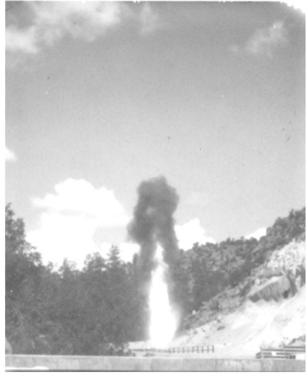
Fig. 6. Photograph showing a Surtseyan jet from Type IV design. The incandescent jet reaches about 15 m high with a dark smoke plume extending above it. The flaring shape of the jet indicates that it is overpressured.
