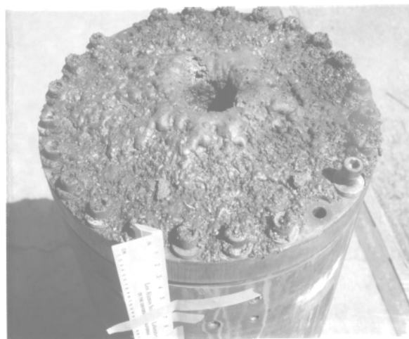
Fig. 1. Photograph of thermite flows extruded on the top surface of the experimental vessel. The surface is about 40 cm in diameter, and the vent is about 10 cm in diameter.
