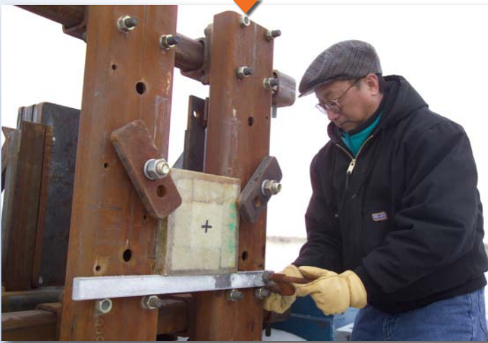
An INL materials scientist prepares a sample of ceramic composite vehicle armor for ballistics testing.
